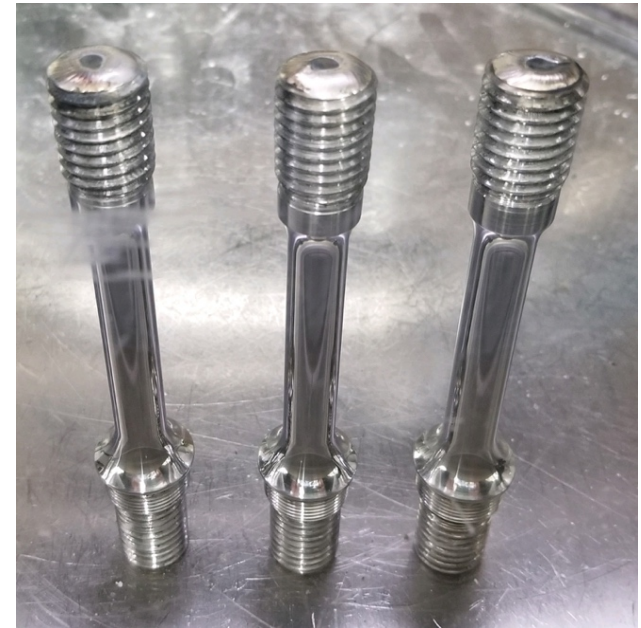
Preparation of RAFM steel tensile specimens for liquid Li embrittlement test B. Pint, J. Jun, ORNL
